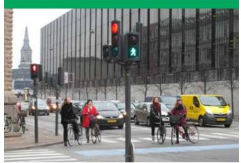
In Denmark, two-stage turns mean cyclists aren't forced to wait in the middle of often intimidating junctions. Minor changes to existing practice would be needed to allow this in the UK.
